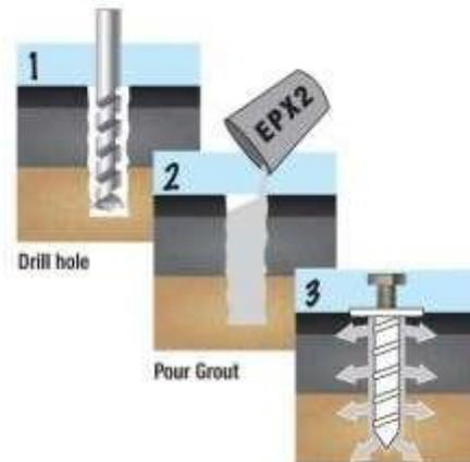
1. Drill a hole per anchor specs
